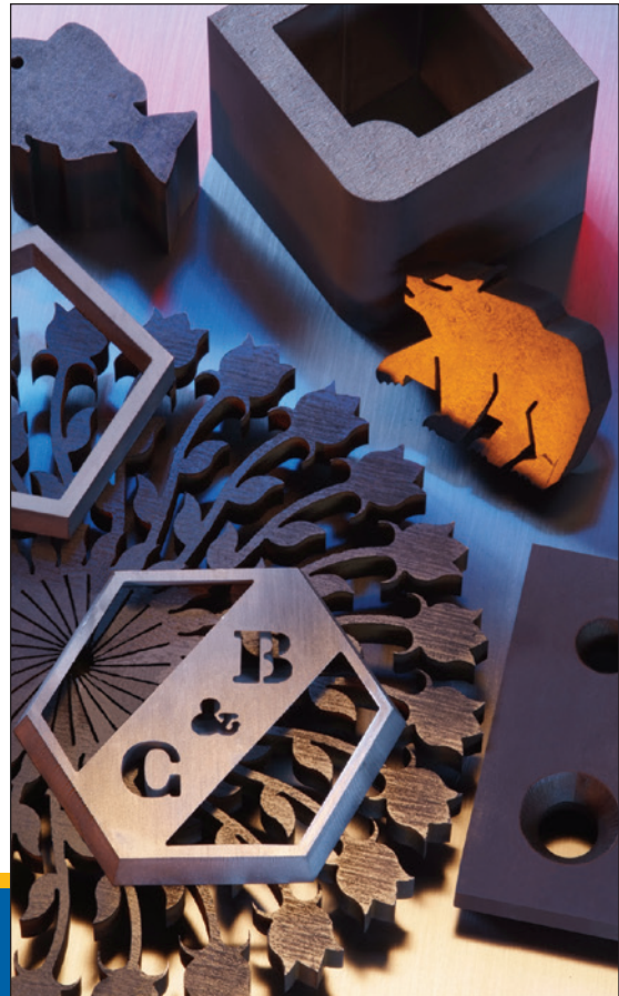
A few examples of some of the zero taper intricate parts that can be achieved with the Dynamic XD Waterjet.
