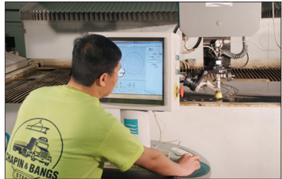
All Waterjet functions are controlled from the digital console.
