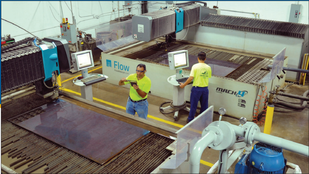
The dual Dynamic XD Waterjets cut any material with virtually zero taper (.001).
